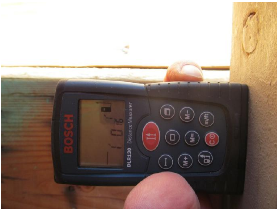
PK-01.051; 11/04/2014; Building 6; Roof Access; Distance of the metal step ladder outside edge to adjacent framing at the top \pm 12 \frac{1}{16} ". See A/2 and A/1.
