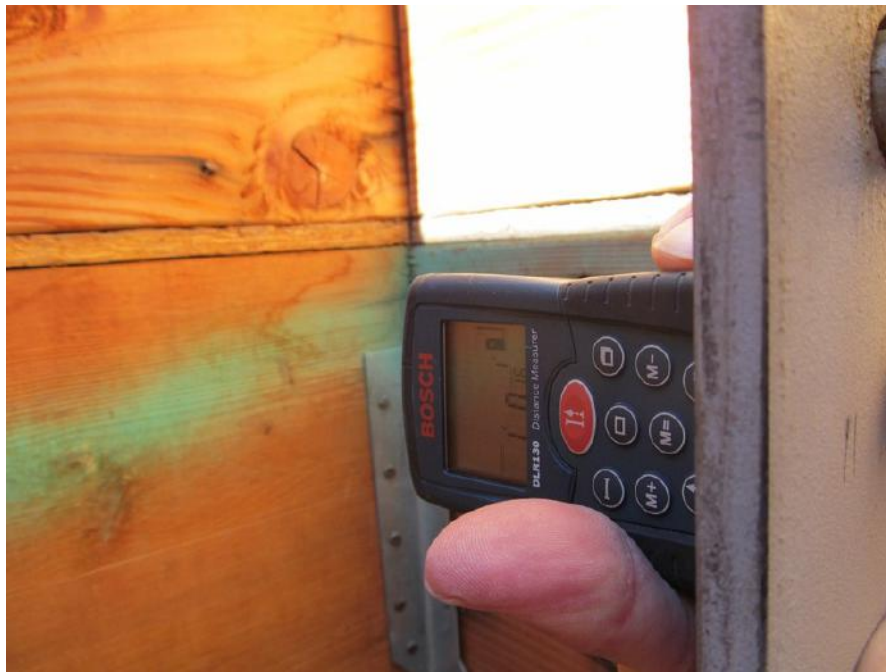
PK-01.052; 11/04/2014; Building 6; Roof Access; Distance of the metal step ladder outside edge to adjacent framing at the top \pm 12 \frac{1}{16} ". See A/2 and A/1.
