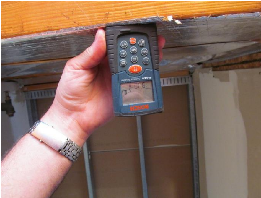
PK-01.025; 11/04/2014; Building 6; Roof Access; Bottom of structural joist at ± 9' - 10 5/8" above the slab on grade concrete below. See A/2.
