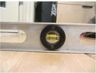
same condition in kitchen). Floor levelness does not conform to industry standards. High point is linear from entry to main living area. Separation noted at wood floors, between planks.
